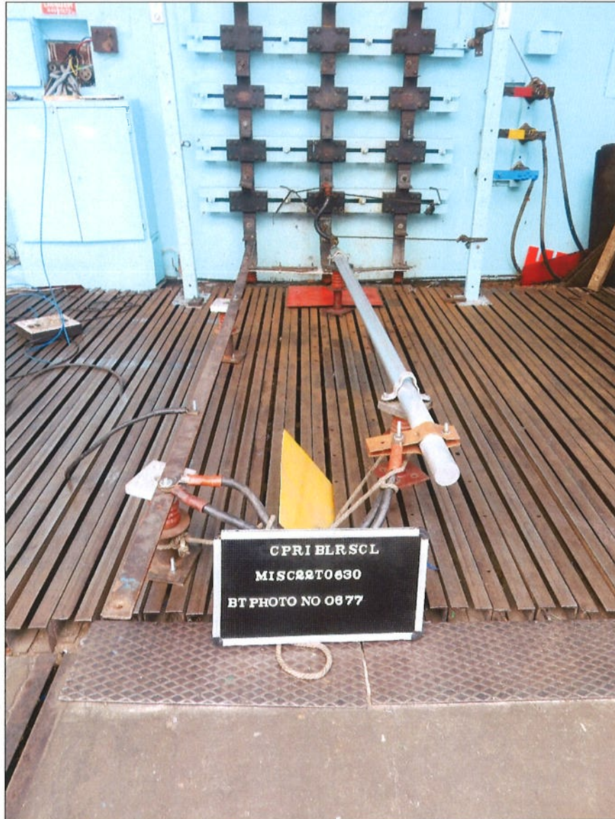
Mounting arrangement (Before test)
